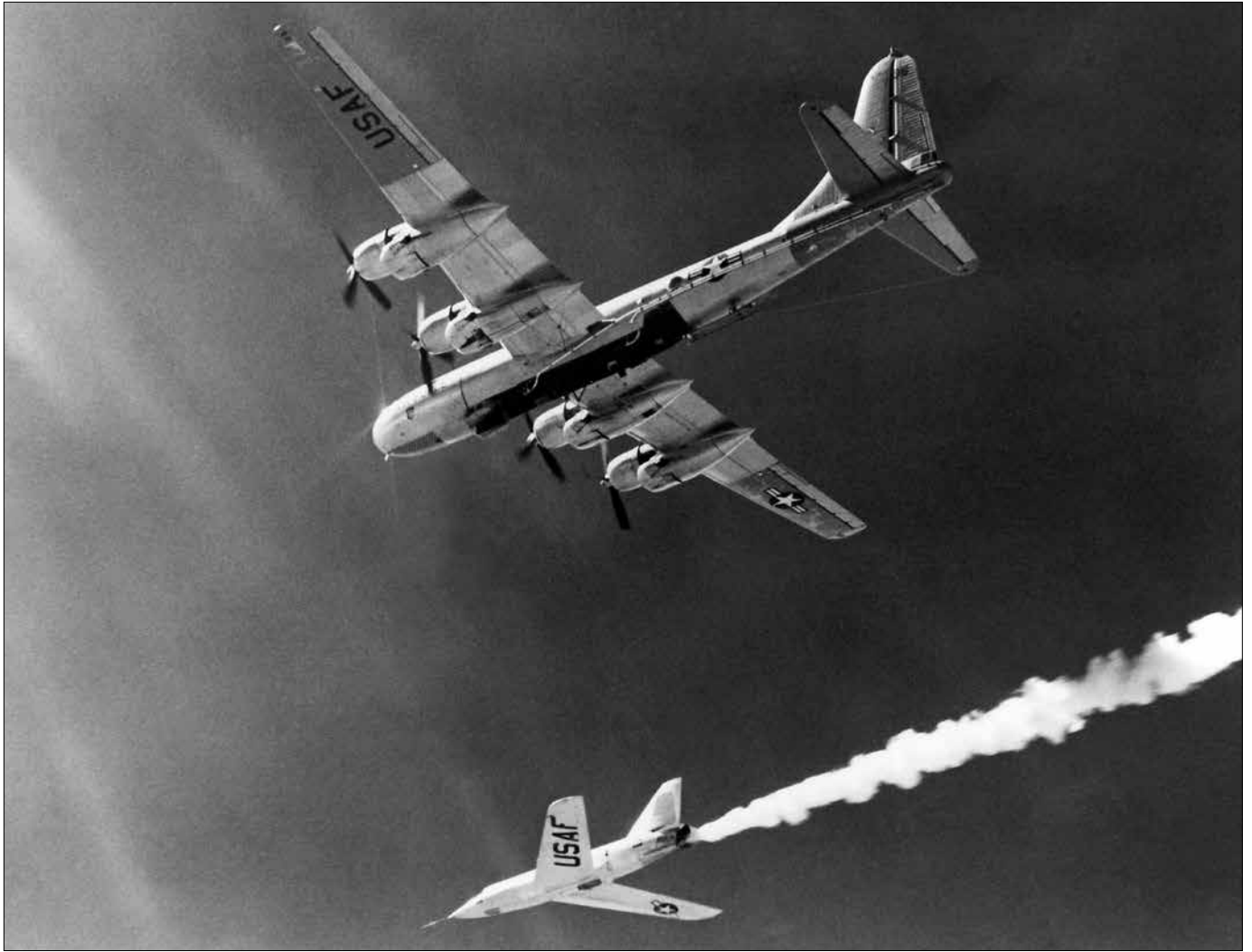
X-2 rocket plane dropped from B-50 Superfortress mothership in mid-1950s (NASA)
